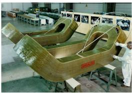
Dipole coils after VPI impregnation
