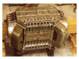
Coils assembled into the cold support
